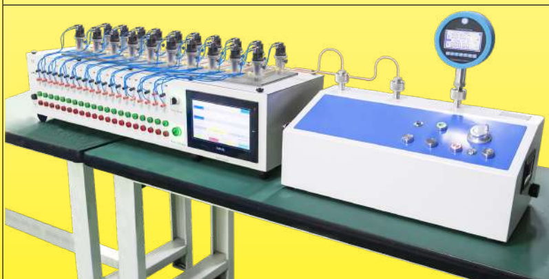
Verification of pressure switch calibration
