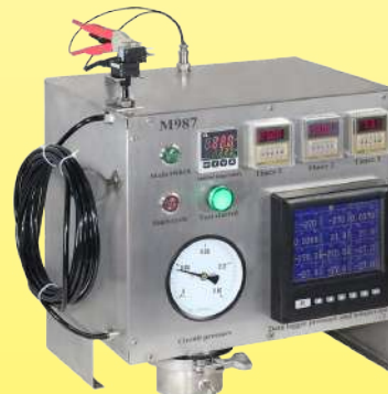
Test equipment for measuring repeatedly and constantly the maximum length of the air switch connecting tubes according to the volume of the push button and the pressure it develops (Ultimheat Laboratory)
